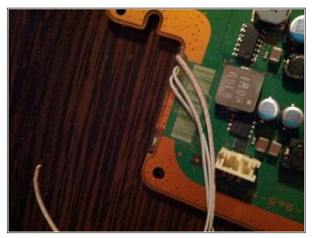
This is the upper side of the Mainboard, you can/should also use some Tape to fix the position of the wires. Also you can see, i glued the connector back on the board (no electrical connection).
