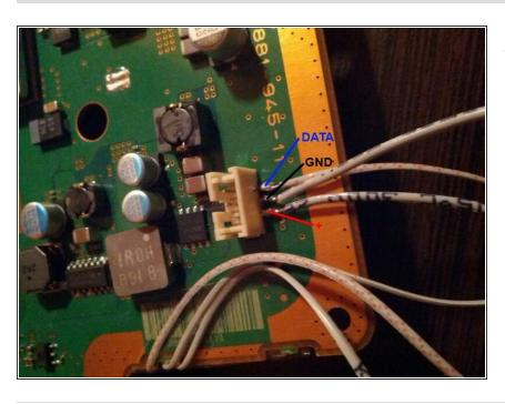
Solder the wires to the Connector you glued on the Mainboard, or directly to the fan or any other idea you can come up with.
