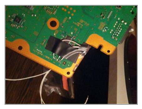
Use some Tape to fix the wires on the Board. As you can see, i used the gap on the right to get the wires to the other side.
