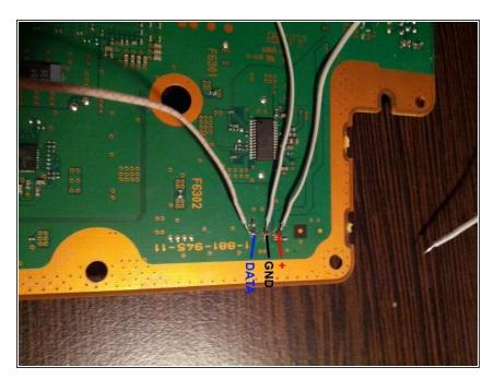
Solder 3 wires to the 3 Points on the Backside of the Mainboard. The 3 Points are right under the Fan Connector on the other side.
