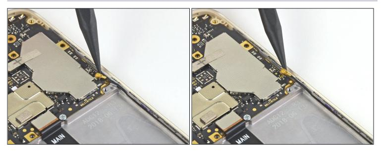
• Use the point of a spudger to pry up and disconnect the antenna cable connector on the motherboard.
