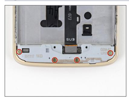
Remove the four 3.8 mm-long Phillips screws securing the daughterboard.
