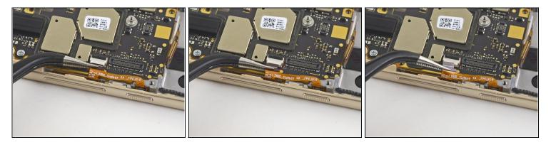
• Use a pair of tweezers to pull the volume button cable straight out of its connector.
