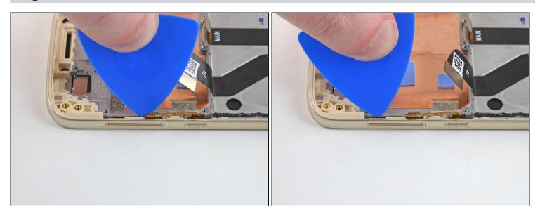
• Slide the opening pick along the volume buttons to cut the adhesive securing it to the phone's frame.
