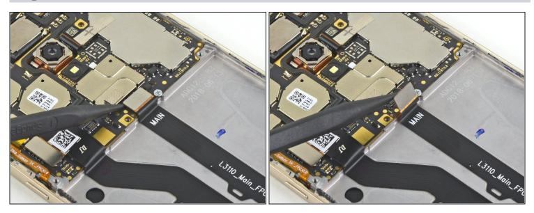
• Use the point of a spudger to pry up and disconnect the daughterboard cable from the motherboard.
