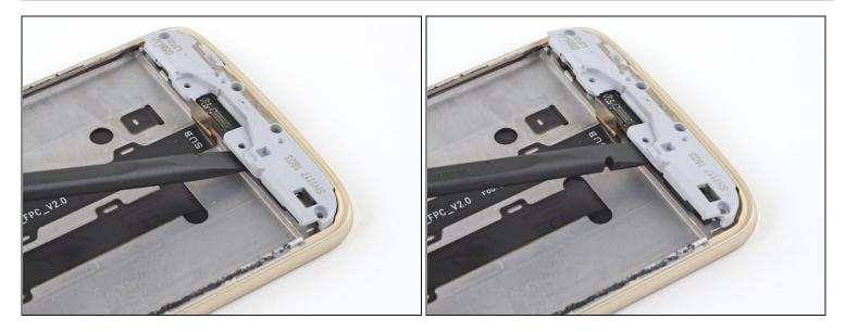
• Use the flat end of a spudger to pry up the daughterboard and free it from its recess.
