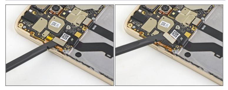
• Use a spudger to pry up and disconnect the display cable from the motherboard.
