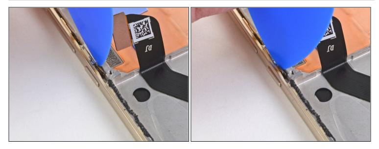
• Insert an opening pick into the gap between the volume buttons and the phone's frame.
