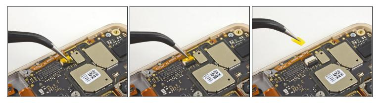
• Use a pair of tweezers to peel up and remove the tape covering the volume button connector.
