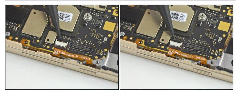
• Use the point of a spudger to flip up the black locking lever on the volume button connector.
