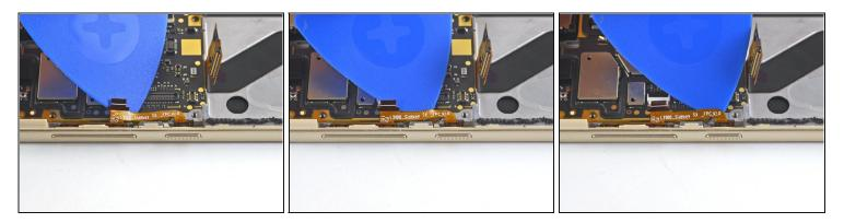
• Slide an opening pick along the underside of the volume button cable to cut the adhesive and free it from the motherboard.
