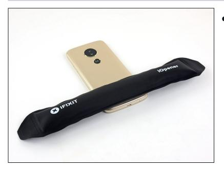
• Use the iOpener to heat the back of the phone along its bottom edge for about two minutes, or until it's slightly too hot to touch.
