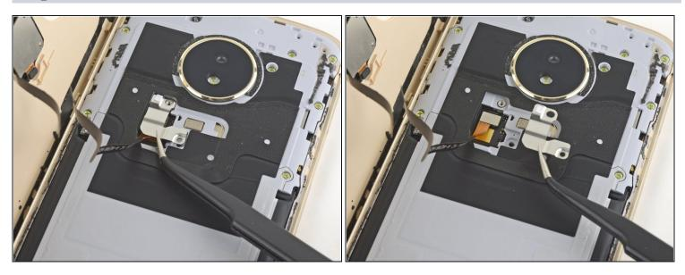
• Use a pair of tweezers to remove the fingerprint sensor cable cover.
