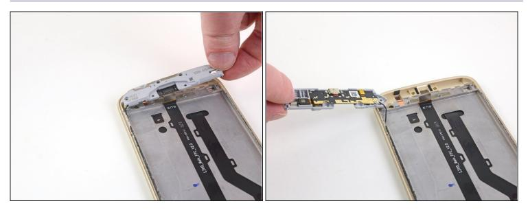
• The daughterboard is still attached to an antenna cable, so lift the daughterboard up from the left side of the phone and flip it over its right side to prevent ripping the antenna cable out.
