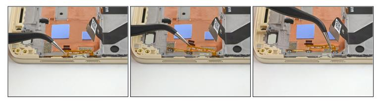
• Use a pair of tweezers to remove the volume buttons from the phone's frame.
