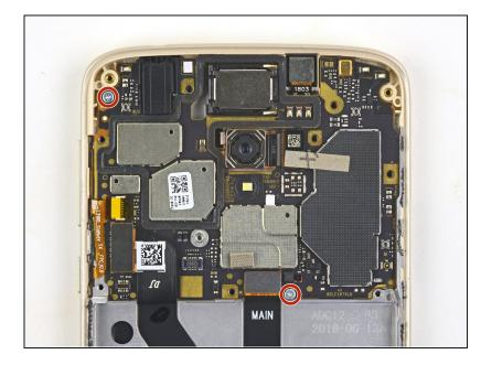
• Remove the two 2.9 mm-long Phillips screws securing the motherboard.
