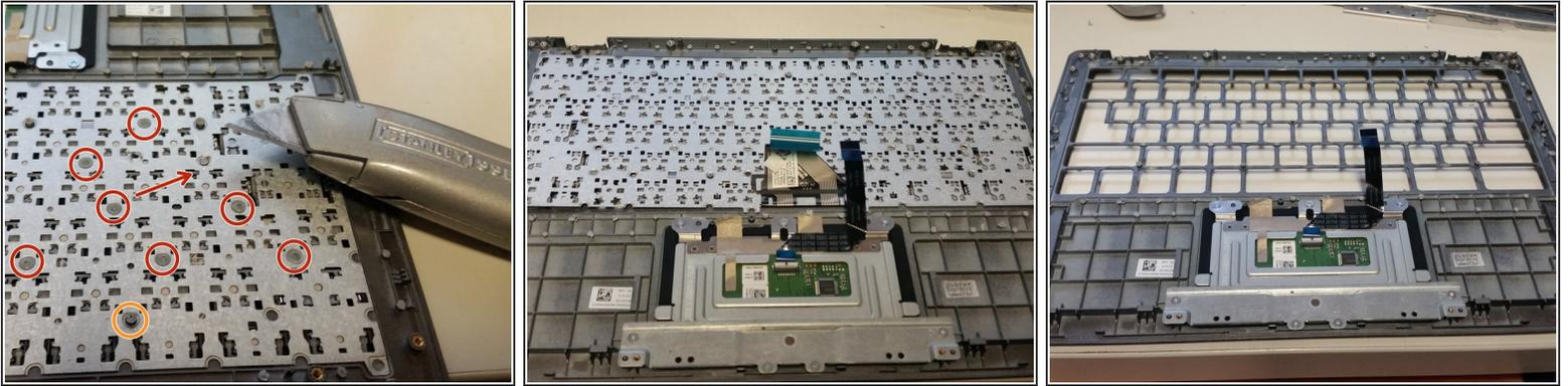
**i** The keyboard is held onto the frame by plastic pins.
