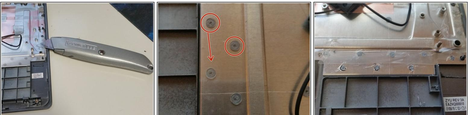
**i** The motherboard plate is held onto the frame by plastic pins.
