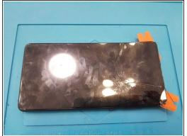
Carefully start to separate the screen as shown. Start from the top corner.
