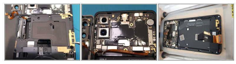
Remove the shield and disconnect the battery connector, LCD and touch connector, and touch ID connector.
