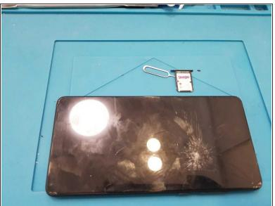
Turn off and remove the SIM card.
