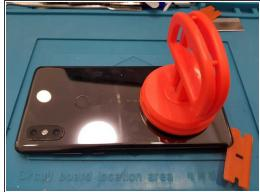
Apply heat to loosen the back cover adhesive. Then remove it carefully.
