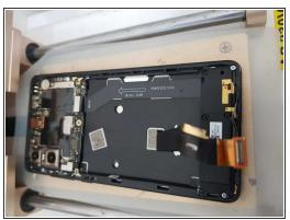
Remove the battery carefully as shown and apply heat to loosen the adhesive holding the screen.
