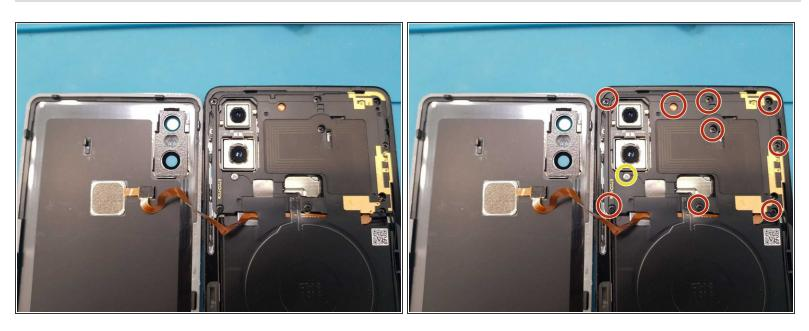
Remove all nine screws that hold the shield protecting the motherboard.
