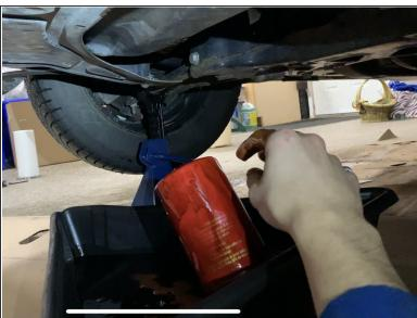
Place old oil filter upside down on the knob in the oil drip pan
