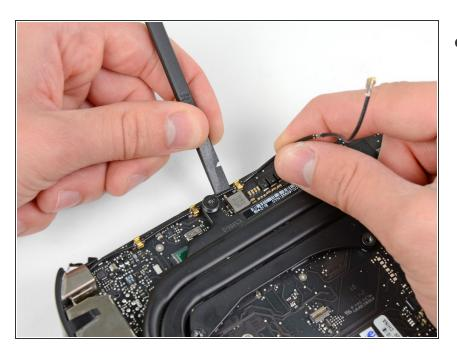
• Carefully un-clip the antenna from the logic board near the heat sink.
