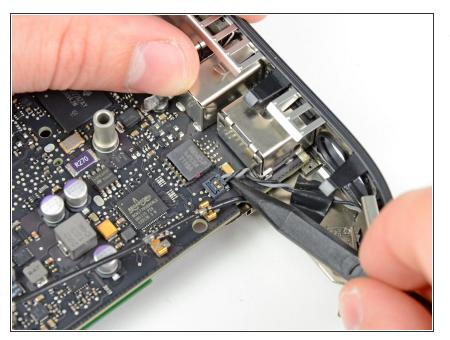
Lift the power button cables upward to gently pull the power button cable up and out of its connector on the logic board.
