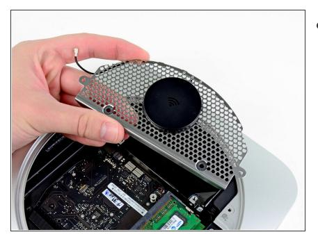
Remove the antenna plate from the mini.
