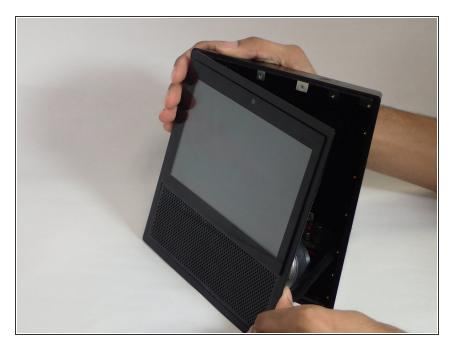
After the screws are removed, grip the front panel and remove, using a plastic opening tool if necessary. This will expose the inside of the device.
