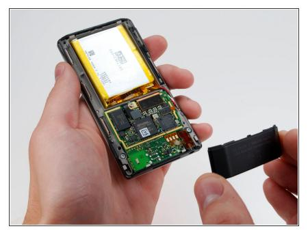
• Removing the bottom backplate.
