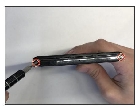
Remove the two 7mm screws holding the back panel of the phone using the P5 bit and magnetic driver.
