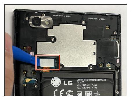
Carefully use the plastic opening tool to pry the ribbon cable connecting the battery to the motherboard of the phone.
