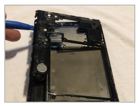
Carefully use the plastic opening tool to pry the plastic shield from the motherboard. This will expose the motherboard and ribbon cables for each component.
