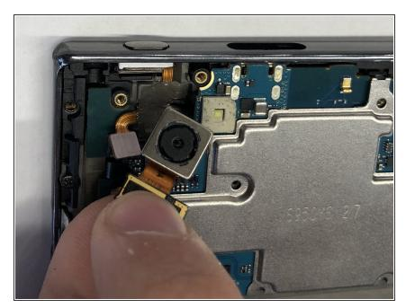
Using the ribbon beneath the camera lift it upwards and pull the camera out.
