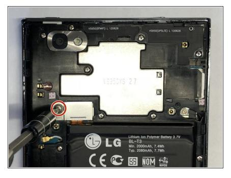
Use the Phillips #0 screwdriver to remove the 5mm screw holding the metal bracket that protects the battery's ribbon cable.
