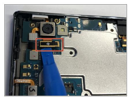
Carefully use the plastic opening tool to pry the ribbon cable below the camera itself from the motherboard.
