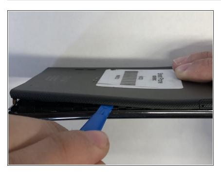
Carefully use the plastic opening tool to pry the back panel of the phone from the front screen. This will expose the battery and other parts.
