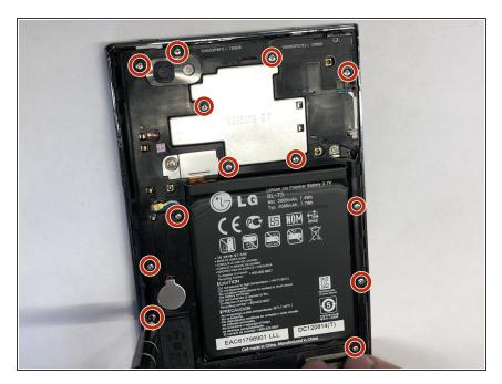
Remove the thirteen 5mm screws holding the plastic shield covering the motherboard using the Phillips #00 screwdriver.
