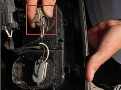
Locate the top light bulb on the back of the tail light casing. This is the bulb you are going to replace.
