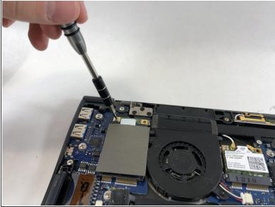
Remove the two 2.5mm Phillips #000 screws at the top of the SSD.
