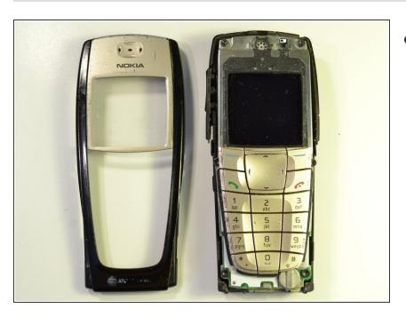
The keypad and LCD screen are revealed.
