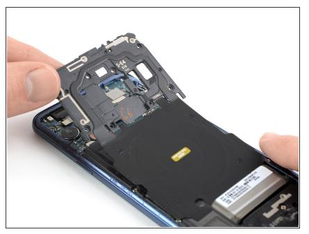
• Remove the plastic cover containing the NFC antenna and charging coil.
