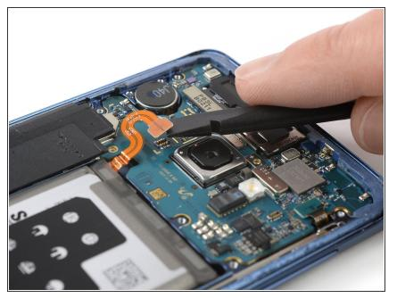
• Use the flat end of a spudger to pry up and disconnect the battery flex cable.
