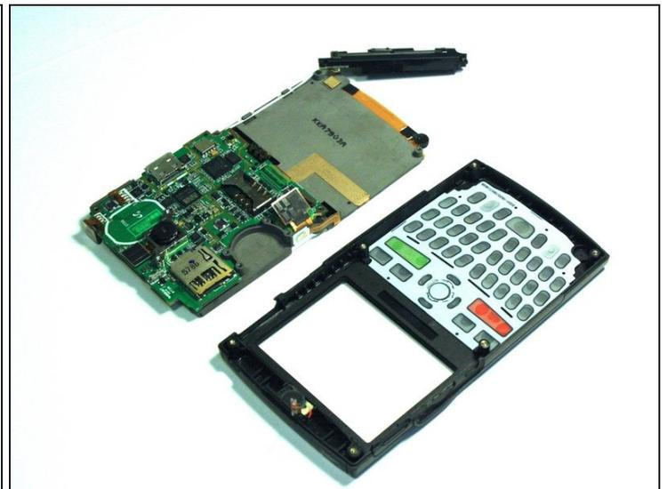
ⓘ Once all of the connections have been snapped off of the motherboard, the motherboard can be removed.
