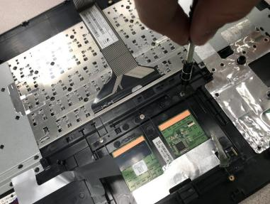
• Unscrew the three 4mm screws on the touch pad with a PH00 screwdriver.
