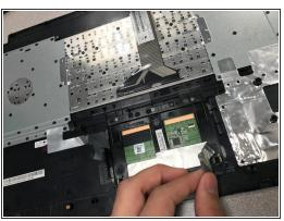
Peel off the silver stickers that are attaching the touch pad to the back part of the keyboard.
