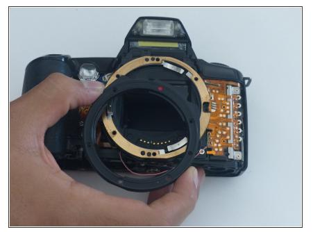
Simply using your fingers - although you can use something else such as tweezers - remove the first layer of the lens mount. This first layer is black, plastic, has a red dot at the top, and so on.
