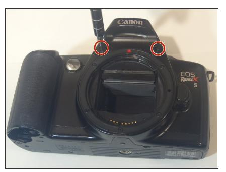
Using a PH000 screwdriver bit, remove the 2 black screws circled in the picture, which are both 6 mm in length and 1.25 mm in diameter.
