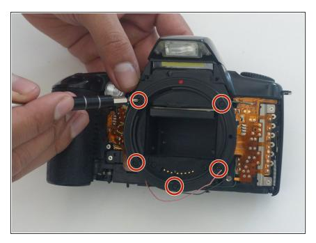
Using a PH000 screwdriver bit, remove the 5 black screws circled in the picture, which are all 5.5 mm in length and 2 mm in diameter.
