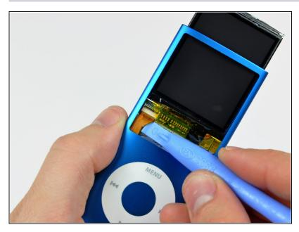
Use an iPod opening tool to peel the display data cable off the thin metal plate attached to the display.
