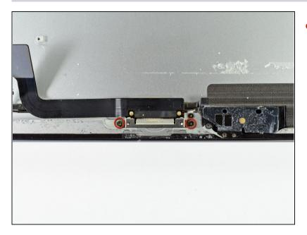
Remove the two 1.8 mm Phillips #00 screws securing the dock connector to the rear aluminum case.
