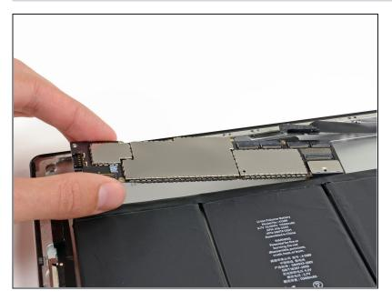
• Remove the logic board from the rear case of the iPad.
