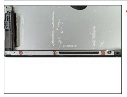
• Remove the three 4.25 mm Phillips #00 screws securing the speaker to the aluminum frame.
