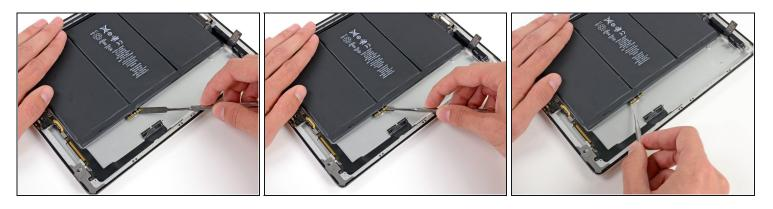
• Carefully slide the metal spudger underneath the battery connector, releasing the adhesive securing it in place.
