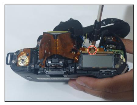
Using a PH000 screwdriver bit, remove the tiny silver screw circled in the picture, which is 2 mm in length and 1 mm in diameter.
