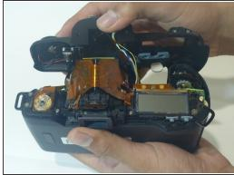
Using an opening tool (you can also use your nails, but try not to use something potentially damaging to the camera such as metal), separate the top cover from the rest of the camera!
