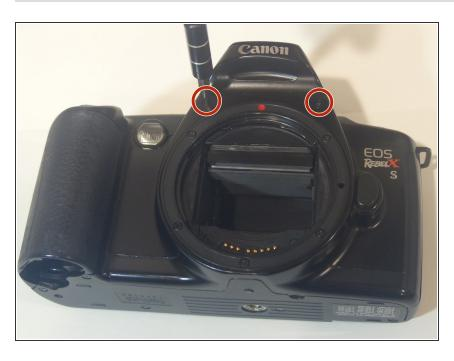
Using a Phillips #000 screwdriver, remove the two black screws shown in the picture that are both 6 mm in length and 1.25 mm in diameter.
