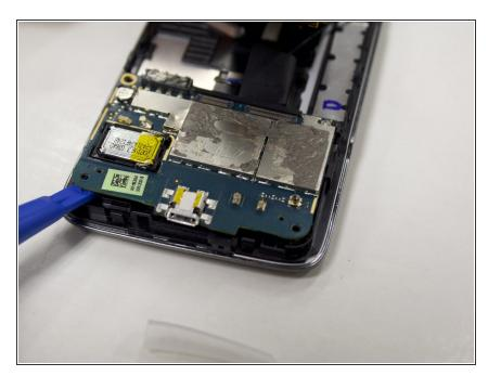
After you remove the ribbon, insert the plastic opening tool underneath the lower motherboard until it is released from the bottom of the device.
