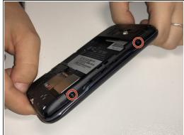
Using a Phillips #00 screwdriver, remove the screws as directed.
