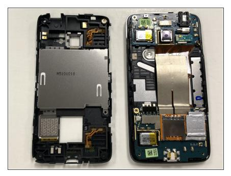
Separate the screen and back cover with the opening tool.
