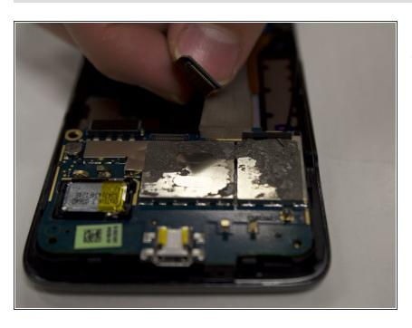
You will notice a ribbon that connects the upper and lower motherboard together. With your fingers, carefully pull up both ribbons that are attached to the lower motherboard.
