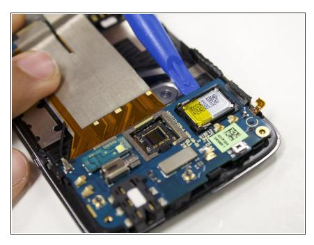
For you to remove the upper motherboard, insert the plastic opening tool underneath the upper motherboard until it is removed from the bottom of the device (same as in step 2).
