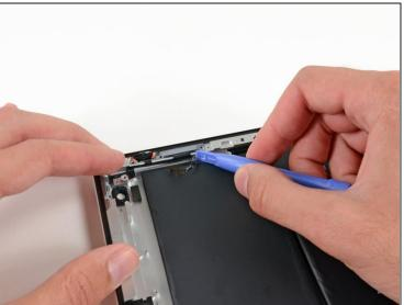
• Continue sliding the plastic opening tool underneath the power & volume cables, releasing the adhesive.
