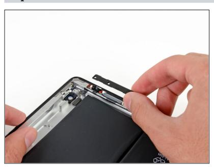
Remove the piece of plastic covering the volume buttons.
