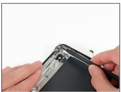
• With the tip of the spudger still underneath the ribbon cable, gently lift the power button out of its socket in the aluminum frame.
