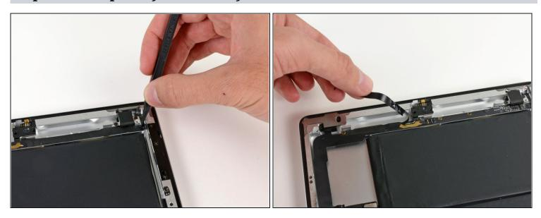
• Peel back and remove the adhesive tape covering the headphone jack assembly.
