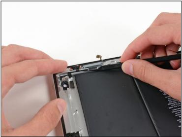
• Using the tip of a spudger, release the adhesive underneath the volume button branch of the ribbon cable.
