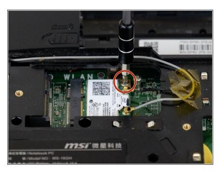
Using a Phillips #00 screwdriver, remove the one 2 mm screw that is holding the wireless card in place.
