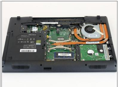
Once all four screws are removed, lift the back off.
