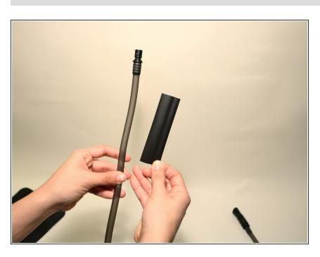
Slide the heat shrink tube over the pipe and hold tightly in place over the ruptured area.
