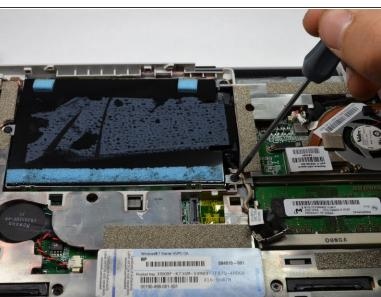
Using a #00 Phillips screwdriver, unscrew and remove the three 2.0 x 4.0 Phillips screws holding the hard drive in place.
