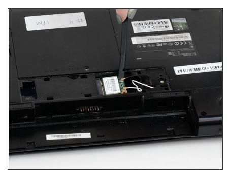
Gently remove the two wires attached to the Wifi card by using a plastic opening tool or plastic spudger to pry up from under where the wire is attached.
