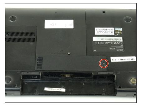
Using a Phillips #1 screwdriver, remove the 5 mm screw located beside the Wifi symbol.
