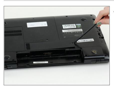
Gently pry up cover using a plastic spudger or opening tool.
