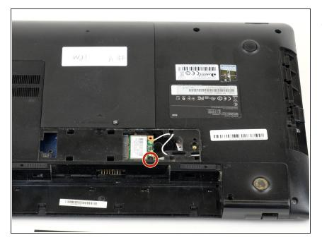
Using the Phillips #0 screwdriver, remove the M2.5x3 mm screw holding in the Wifi card.
