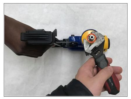
Using a crescent wrench, loosen the yellow nut located between the grip and the male air compressor adapter.
