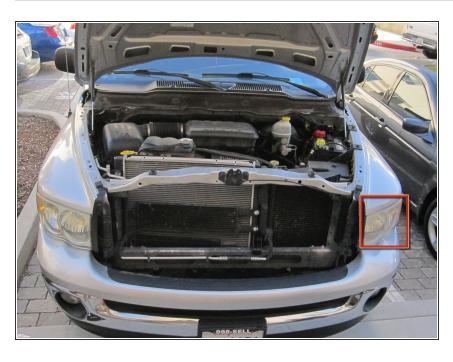
In this guide we will be removing the left headlight. The steps are mirrored for the right headlight.
