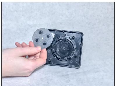
Remove the rubber pad from the joystick.
