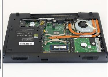
Once all four screws are removed, lift the back off.
