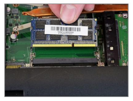
Slide the RAM out of the slot carefully.
