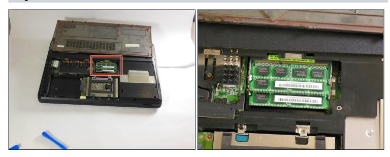
• With the underside plate removed, you can easily access a few RAM chip slots. These are the ones most likely filled with RAM chips from the factory when purchased at retail.
