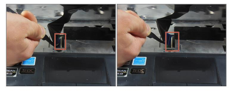
Just above the trackpad, there is a second, wider ribbon cable connected to the motherboard. Unplug this cable.
