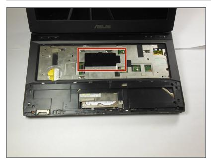
i If you want to add additional RAM, more ports can be found underneath the black plastic flap on the top side of the laptop, just under the keyboard. These ports behave the same way as the ones on the backside of the computer.
