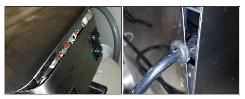
• Replace the cover, making sure the steel lip at the front is in its slot, and that the black plastic bushing is in place at the back of the cover. Replace two of the six screws, to save time in case you have to repeat the process.
