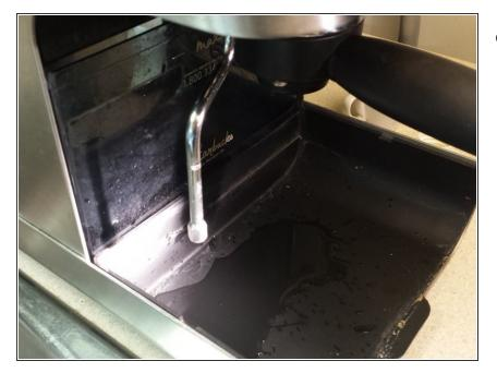
When there is water leakage from the steam valve, there are 2 sources, external and internal.
