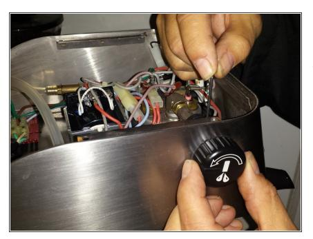
• Now, while bracing the hex wrench, turn the steam valve knob slightly in a clockwise direction, perhaps 1/8th of a turn or less. This is compressing the seat of the steam valve plunger to close off the water leak when the machine is on.
