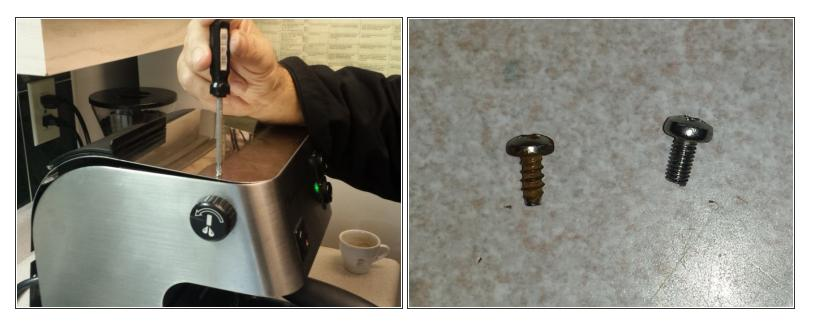
Remove the six screws holding down the cover. Note that the top screws have fine threads, while the four lower screws have coarse threads. Keep this in mind for later reassembly. Once the screws are off, remove the cover.
