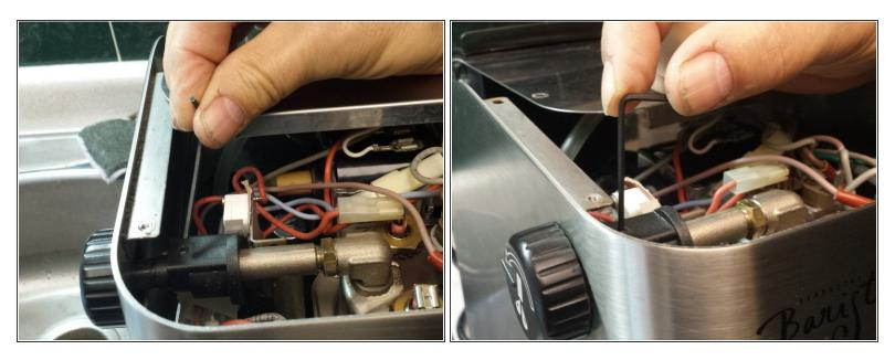
Note where the steam valve knob connects to the valve assemble, at the top is a small hex nut. Use the 2mm hex wrench to loosen the nut by turning it counter clockwise, about 1/4 turn. Hold on to the wrench, keeping the steam knob shaft in the upright position.
