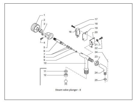
If the steam wand is still leaking after a second try, then the steam valve plunger needs to be replaced. This is part number 8 on the schematic. Overhaul kits can be acquired from sources like espressocare.com. You can follow the tear down instructions on this site, or some of the video sources on youtube.com.
