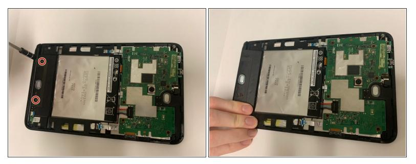
Unscrew the two screws of the plastic piece, and lift it off.
