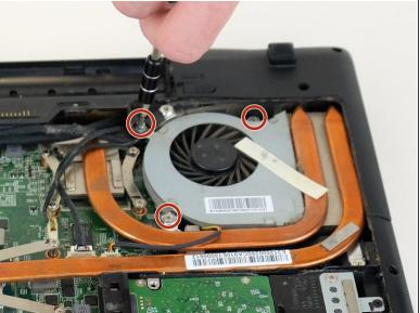
Remove the three 5 mm screws from the fan with a Phillips #00 screwdriver.
