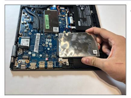
• Lift the hard drive up and out.
