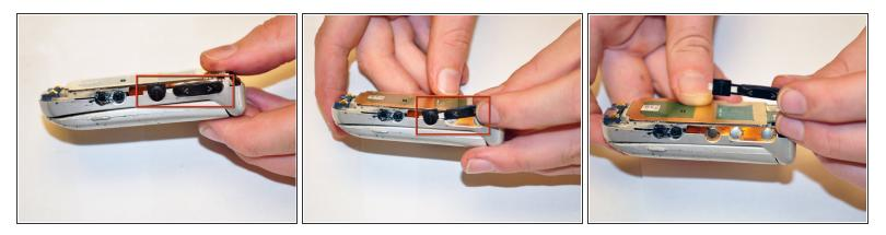
• With the back case fully removed and out of the way, use your fingers to remove the volume button.
