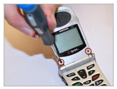
Use a Philips #0 screwdriver to remove the two screws below the screen.
