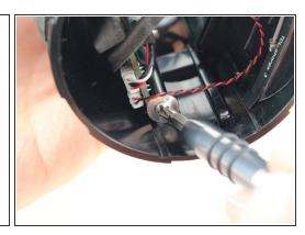
Remove the two 9mm Phillips #1 screws holding in the sides of the motherboard.
