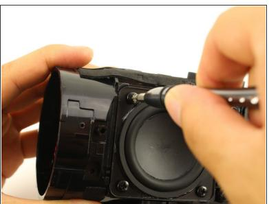
Remove the eight 10mm Phillips #1 screws from around the two front speakers.
