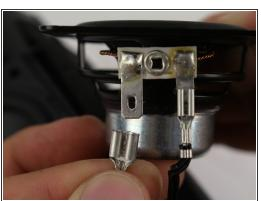
Press the small metal tab on the speaker connector with a Phillips #000 screwdriver and gently pull the connector apart.
