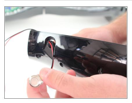
Pull the power button through the hole in the shell.
