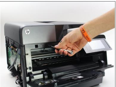
Remove the 11.6mm T9 screw from the top left of the front of the printer.
