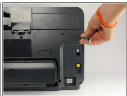
Remove the two 11.6 mm T9 screws from the right side of the back of the printer.
