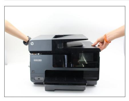
Remove the top of the printer by lifting it from both sides.
