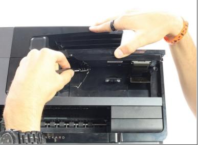
Remove the two 11.6 mm T9 screws from beneath the display.
