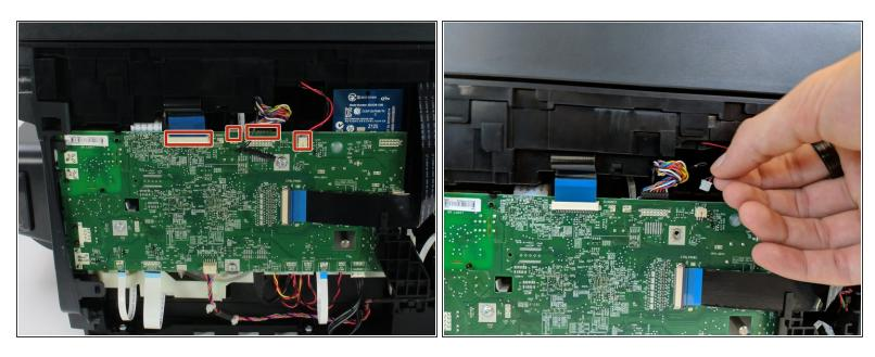
Remove the four connectors from the top of the motherboard.
