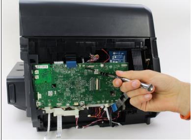
Remove the one 5.3 mm T9 screw.
