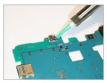
Use the soldering tool to remove the charging port. To reassemble your device, follow these instructions in reverse order.
