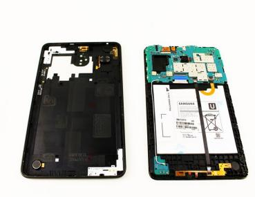
Use the iFixit Opening Tool to pry off the back case, moving the tool around the screen.
