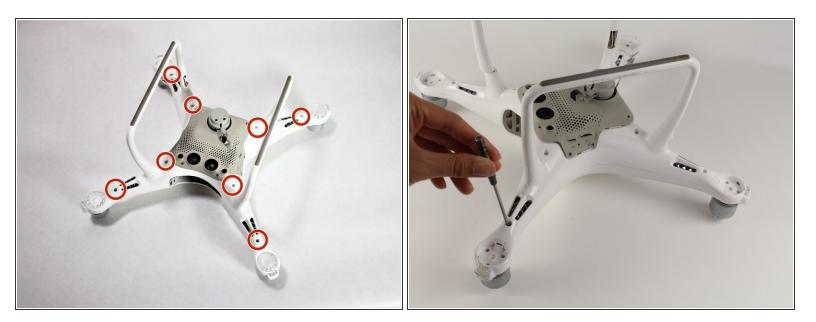
• Remove the eight 7 mm hex screws by turning counterclockwise with a 2 mm hex bit.
