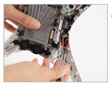
Unlodge the glue from the board using a metal spudger.
