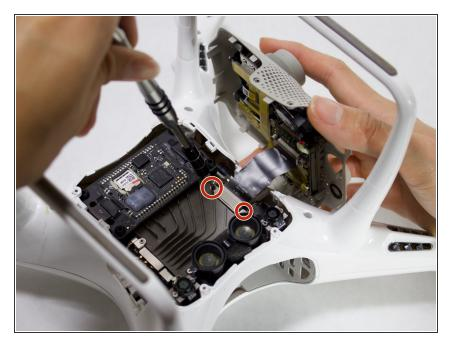
Remove two 1.2mm screws using the JIS #000 bit from the camera cable retaining bracket.
