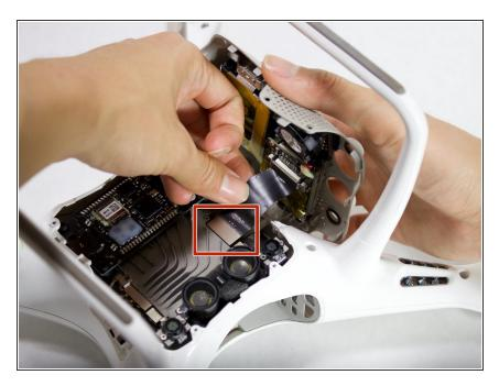
• Lift the camera connector at one end with your hand and remove the mesh.
