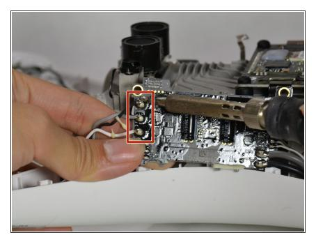
Desolder the motor and LED wires on both sides of the board. For general soldering information, visit this <u>Soldering Technique Guide</u>.
