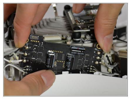
• Jiggle the electronic speed controller board up and away from the drone.
