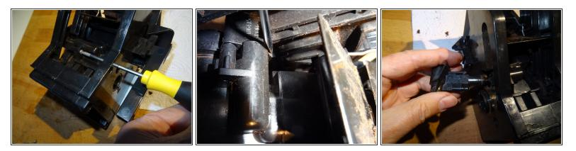
• Through the hole on the opposite side of the fixing screw can be solved. The inlet is plugged in and held by a latch, which you have to push away.
