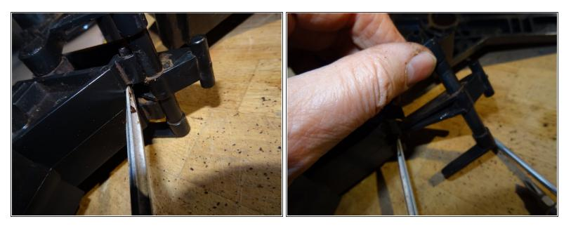
That's the trickiest part: you have to lever this lever out of its camp. To do this you drive with a screwdriver between the lever and the carrier and press it really very strong outwards. Now he grabs out - hopefully!
