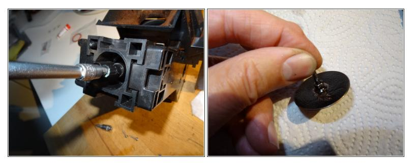
• With a 6mm Allen key (or the key that comes with the machine), the brewing sieve can be unscrewed. It strongly determines the aroma, if it is dirty the coffee tastes bad.
