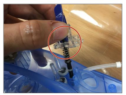
Pull out the settings switch for the clothes iron, this is very easy as it is not held in place by any fasteners.
