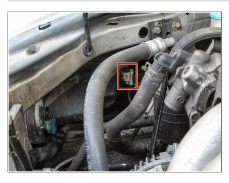
Identify your lightbulb hardware. This can be easily done by looking directly behind the light bulb for a white plastic headlight clip that houses both a wire and piece of hardware that feeds into the headlight housing.
