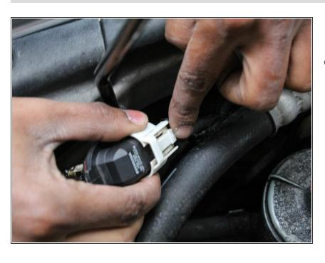
Remove the lightbulb that needs replacing from the white plastic piece by pressing down on the tab that is located on the bottom of the piece. While pressing down, slide the lightbulb outwards to remove it.
