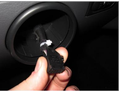
Slide the connector back into the housing and replace the zip tie you cut earlier.
