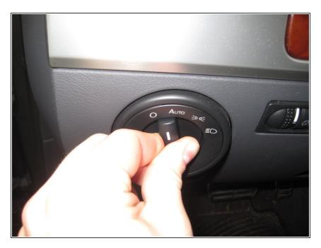
While keeping it depressed, rotate the switch to the right. It will turn slightly.
