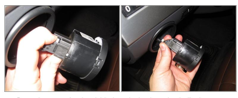
Remove the connector from the switch by depressing the release tab and pulling the connector out.
