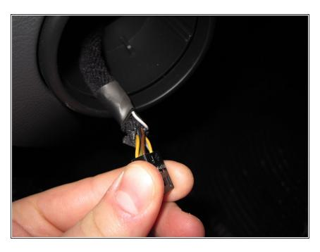
Now fold the wire back up against the harness and use the electrical tape to hold it in place.
