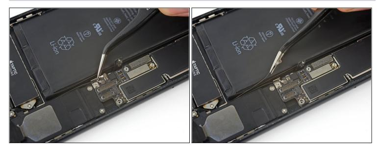
• Carefully de-route the coaxial cable you just disconnected from the small metal clip holding it to the logic board.
