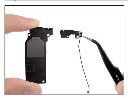
Remove the Wi-Fi diversity antenna from the speaker. Compare your new replacement part to the original part—you may need to transfer remaining components or remove adhesive backings from the new part before installing.
