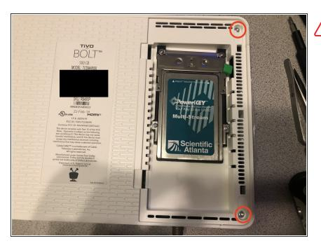
Do not attempt to remove the housing yet. Still 3 more screws and plastic clips holding it in place
