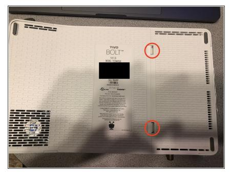
Undo the clips to lift up the Cable card slot cover
