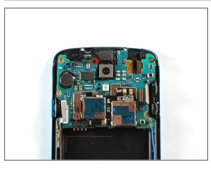
Remove the single 2.4 mm Phillips #00 screw from the motherboard assembly.
